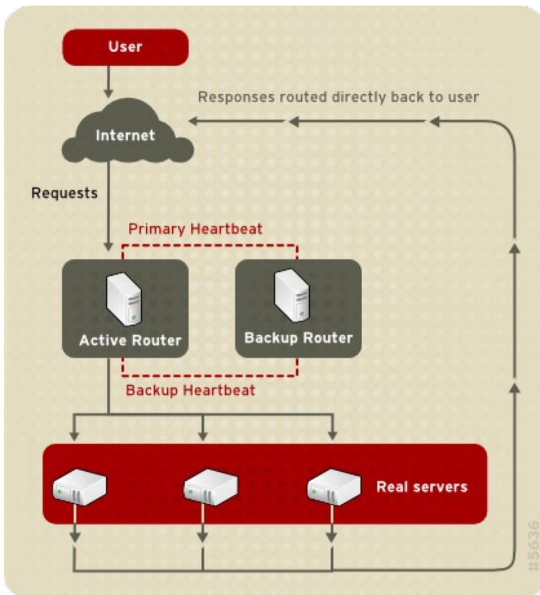
**Figure 1.4. LVS Implemented with Direct Routing**
