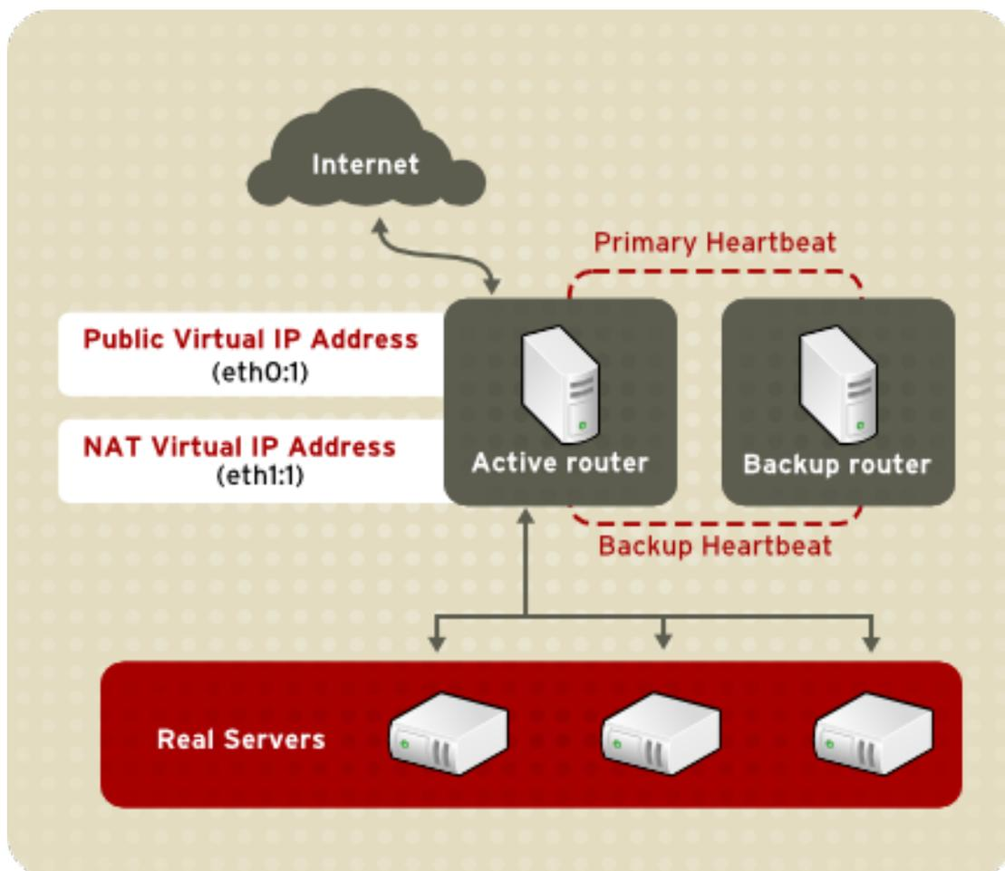
Figure 1.3. LVS Implemented with NAT Routing
