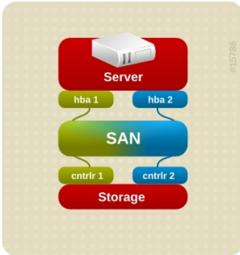
Abbildung 1.3. Active/Active Multipath Configuration with One RAID Device
