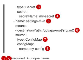
Required. The absolute path of the mount point. It must not contain .. or : and does not collide with the destination path generated by the builder. The /**opt/app-root/src** is the default home directory for many Red Hat S2I-enabled images.
