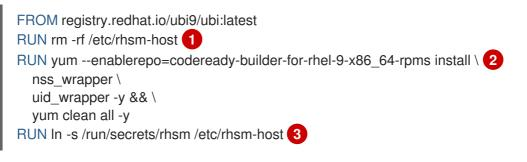
You must include the command to remove the /**etc/rhsm-host** directory and all its contents in your Dockerfile before executing any **yum** or **dnf** commands.
