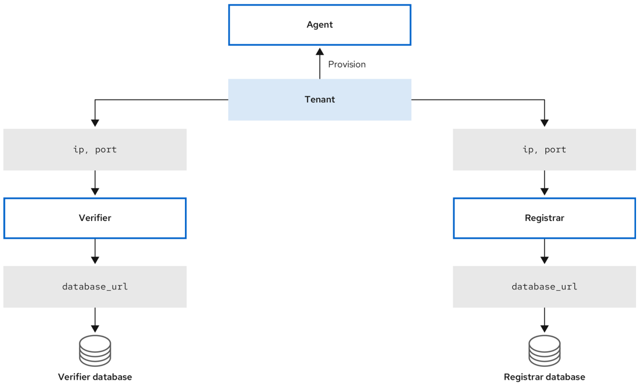
Figure 8.1. Connections between Keylime components through configurations
