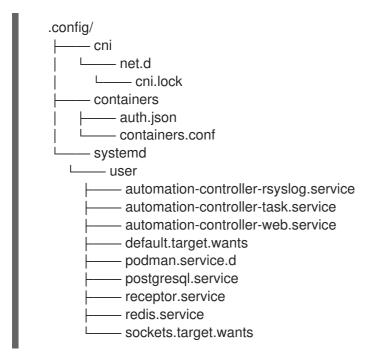
This is specific to Podman and conforms to the Open Container Initiative (OCI) specifications. When you run Podman as the root user /var/lib/containers is used by default. For standard users the hierarchy under \$HOME/.local is used.
